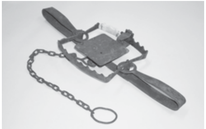
Fig.18. A properly adjusted Lanes trap ready to be attached to an anchor point or drag, and set in the ground.
